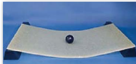
Laminated safety glass made of 2 x tempered glass - both panes broken
